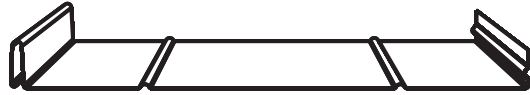
2 Pencil Ribs Profile (1/4" wide) (Disclaimer must be signed for this profile. See below.)
