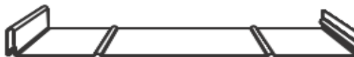
2 Pencil Ribs Profile (see disclaimer below) Note: Pencil ribs are 1/4" in width
