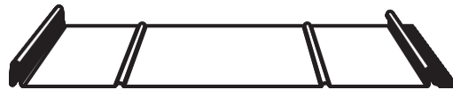
2 Pencil Ribs Profile (see disclaimer below) Note: Pencil ribs are 1/4" in width
