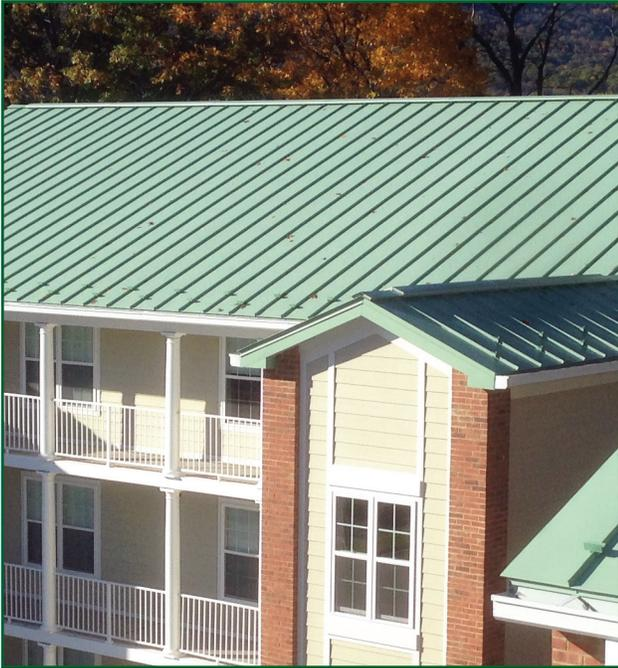
ML150 is a mechanically seamed standing seam panel for architectural applications. The panel has 1.5" high ribs and is secured with concealed clips and the ribs are locked together using a rooftop seaming machine. ML150 can be curved to meet radius panel applications. ML150 is typically specified as an accent feature for schools, shopping centers, banks, hotels, offices, and a variety of other applications.
