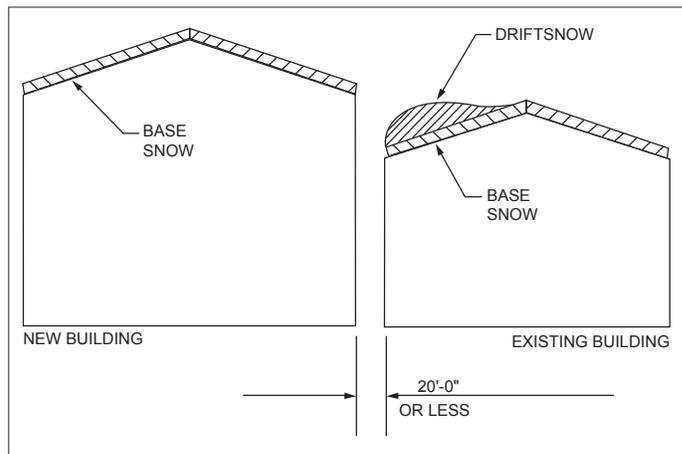
Placing a new taller building adjacent to an existing building can result in snow drift loads on the existing building that were not considered in the original design. The new snow drift load could cause the original building to collapse. When adding a new building within 20 feet of an existing building, the existing building should be checked for potential additional loads and reinforced if necessary.
