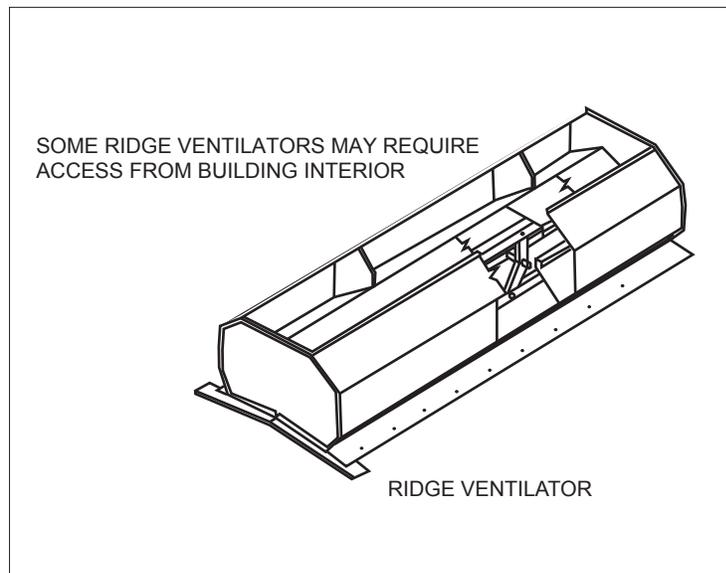
Vents that do not have moving parts will require very little maintenance. Ventilators containing moving parts such as pulleys, rollers or cranks for flue operation will require periodic lubrication at pivot points. Simple operation from time to time will aid in breaking corrosion loose
